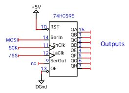
**Input Only Example.** 8-bit General purpose inputs. SS pin used as a latch clock. It must be set up as a general purpose output to transfer the input latch contents to the SR before the data is shifted in. This is a positive edge triggered device so it requires: CPOL= 1, CPHA=0.
